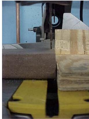
Figure 15: Specimen against board stop for first cut
