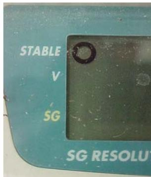
Figure 17: Circle indicates “Stable” weighing condition
