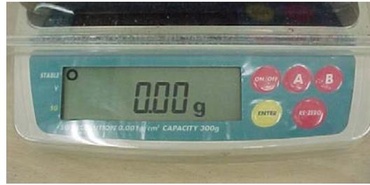
Figure 12: Densimeter in operational mode
