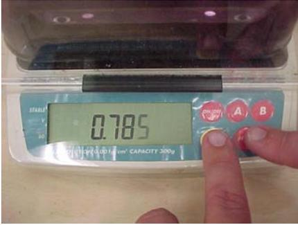
Figure 11: Switch to “ethanol density input” mode
