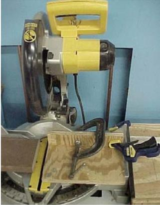
Figure 14: Securing wood board stop using C-clamps
