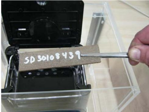
Figure 19: Using forceps to place specimen
