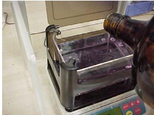
Figure 9: Filling densimeter bath with ethanol to black indicator lines
